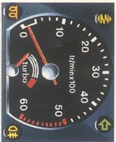
**Tachometer (Diesel engine)**
