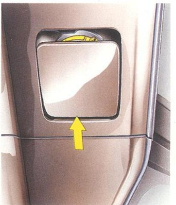
If the central locking fails to operate, unlock the flap by pushing the bolt towards the rear, gaining access through the opening in the boot.
