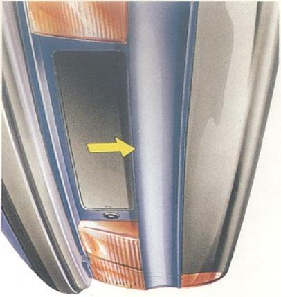
The fuel filler flap lock is operated by the central locking.
