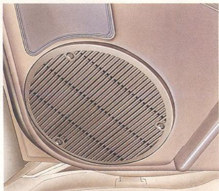
Remove the grille using a screwdriver (see diagram), cut out the panel and the lower half of the inner panel. Connect and secure the speaker. Refit the grille.
