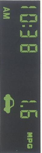
Instantaneous fuel consumption. The fuel consumption of the last 2 second period is displayed. This function is only available at speeds above 13 m.p.h.
