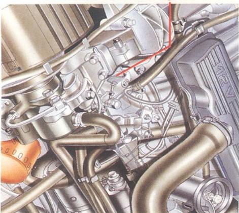
Do not remove the seals on the pump setting screws under any circumstances. Alteration of the settings might lead to early engine failure and loss of warranty cover.
