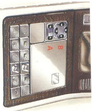
The defrosting of the rear view mirrors is linked to the electrical demisting of the rear window.\*
